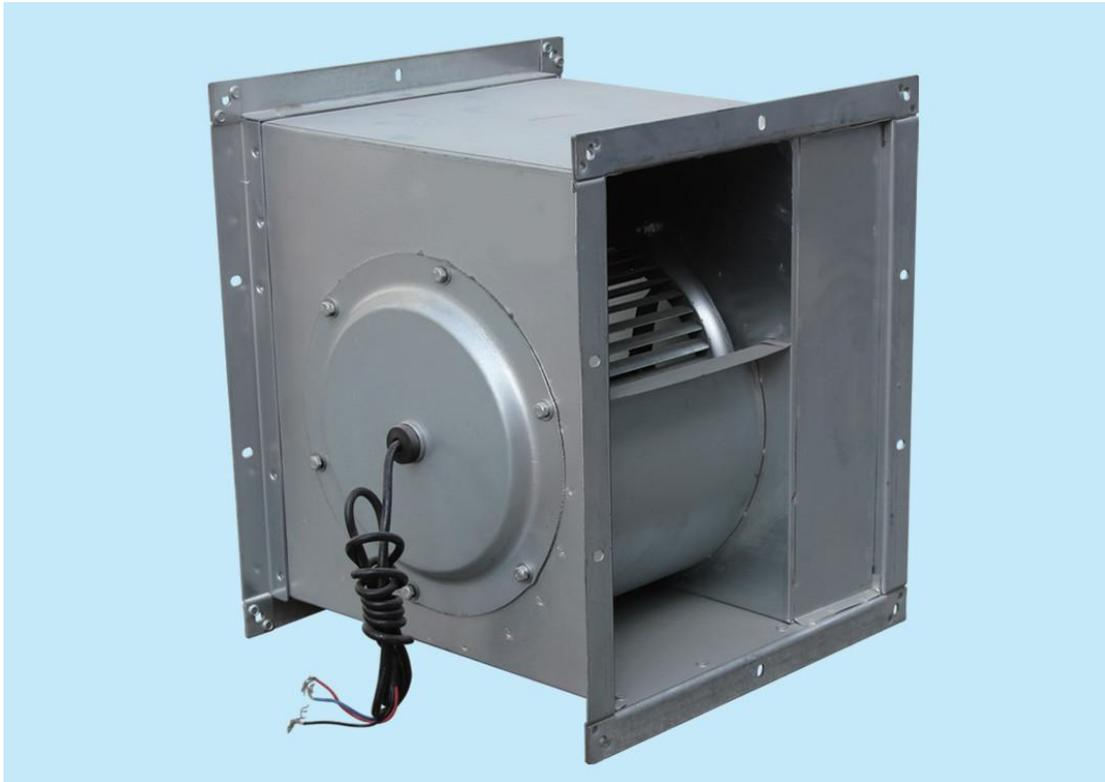
LKWG series duct fan with external rotor motor adopts square inlet and outlet flange. Its shape is similar to a section of air duct. It can be directly installed in the ventilation duct without ground installation foundation. It is very convenient to install, operate and maintain.
