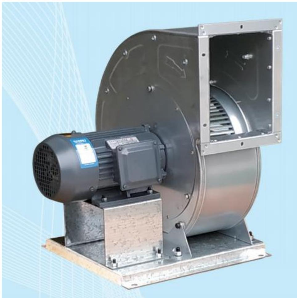
LKZD series forward-curved blade single-inlet shaft-driven centrifugal fan is characterized by that the motor is located at the non air inlet side of the fan, the motor shaft is directly connected with the fan impeller, the motor does not contact with the conveying medium, the structure is simple and reliable, especially suitable for conveying clean gas, dangerous gas or other special gas.
