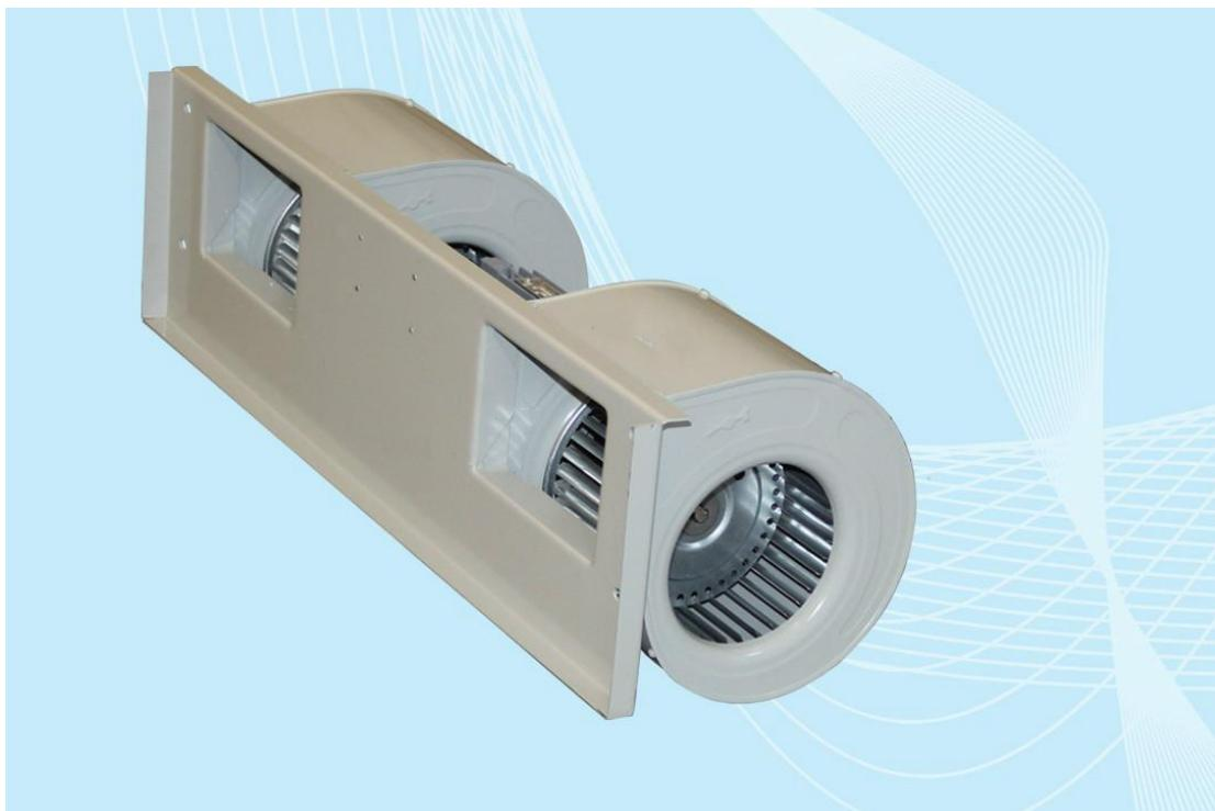
LKZS series double volute forward shaft drive centrifugal fan adopts the special structure that **the impellers of two double inlet centrifugal fans are directly connected to the long shaft of the same motor**, reduces the volume of the whole machine, and can obtain larger ventilation volume under the condition of small installation space.
